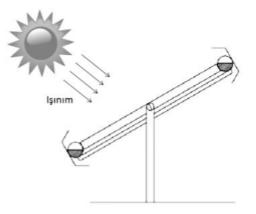
Active followers, on the other hand, can be microprocessor and electro-optical sensor-based, computer-controlled date and time-based, two-faced solar cell-based, and a combination of these three systems.
