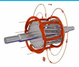
The rotation speed of the magnetic field determines the speed of the rotor. After the rotor starts to rotate with the rotating magnetic field under the influence of the rotating magnetic field, it accelerates and its speed finally becomes equal to that of the rotating magnetic field.
