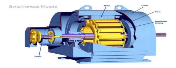
The sections of synchronous motors are the same as induction motors; The stator, which creates a rotating magnetic field through the voltage taken from the three phases, the rotor that performs the rotational movement by interacting with the stator, the cooling fan that undertakes the task of distributing the generated heat, the terminal box where the connections are made and the shaft where the movement is transmitted are the same. caused by its occurrence.
