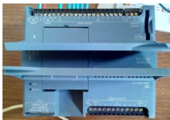
Image 11 CPU – Siemens S7 1200
